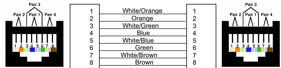
Figure 7 – Wiring Diagram of CAT5 Cable (Direct Type)
