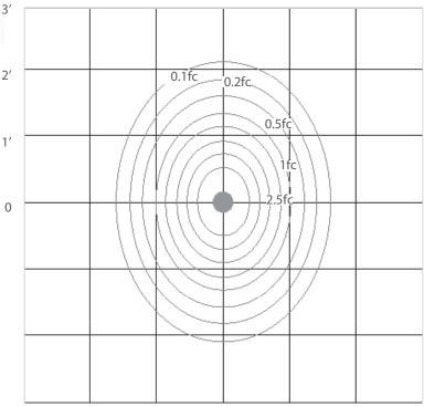
Photometric Performance: Values Based on 610 mm (24") Mounting Height
